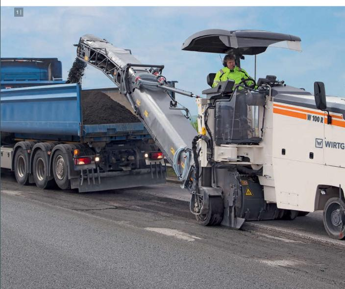
2 The quick-release coupling speeds up the process of mounting and removing the discharge conveyor.
