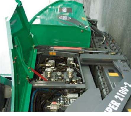
The standardized service concept conceived for the "dash 2" pavers means that servicing is quick and uncomplicated. Large hinged panels provide convenient access to all service points on the machine.
