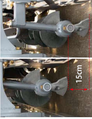
The augers of the SUPER 2100-2 are infinitely variable in height up to 15cm while paving.
