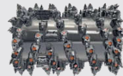
Standard milling drum Milling width: 1,300 mm Milling depth: 0 - 330 mm Tool spacing: 15 mm
