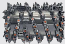
Standard milling drum Milling width: 1,200 mm Milling depth: 0 - 330 mm Tool spacing: 15 mm
