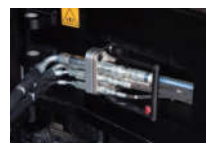
Hydraulic quick coupling system for track motor hydraulic connections
