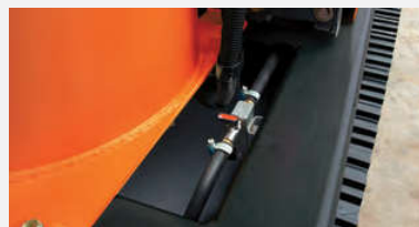
Fuel tank water drainage cock
