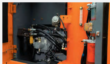
Grouped remote filters and inspection points
