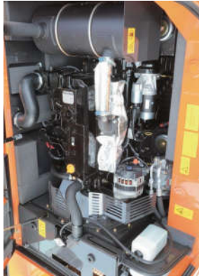
New electronically-controlled engine
