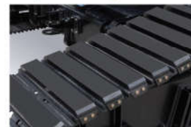
Standard, 3-bar semi grouser shoe
