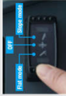
Clutch cut position switch
