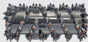
Milling Drum Milling width: 1,800 mm Milling depth: 0 - 330 mm Tool spacing: 18 mm
