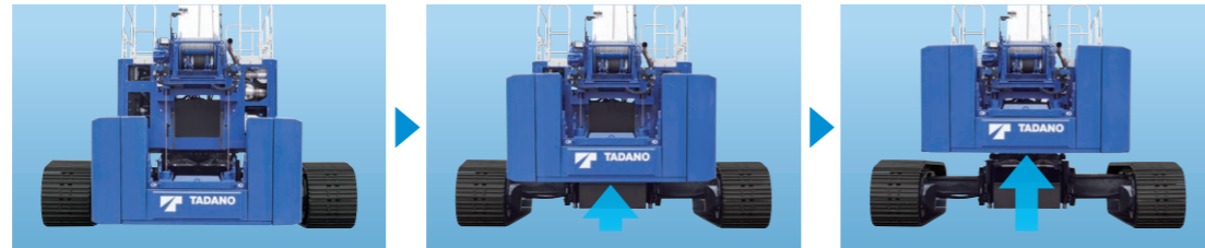
Configuration "A" 10.6 t Configuration "B" 21.2 t Configuration "C" 31.8 t Three counterweight configurations can be selected.
