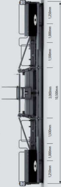
SB 300 TV Built up to maximum pave width with hydraulic bolt-on extensions.
