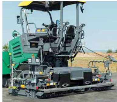
AB 340 with 25cm bolt-on extensions
