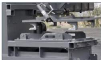
Step 1: Drive up to the side of the offset mould
