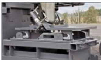
Step 2: Lower the attachment plate with mounting hooks
