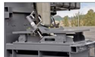
Step 4: Secure offset mould with hydraulic cylinders
