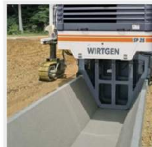
Slipform under the machine (Inset)
