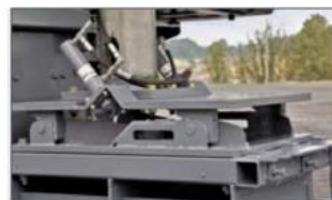
Step 3: Slide the mounting hooks into the guides
